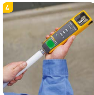
Pin continuity test: Tests if filaments have continuity
